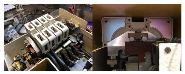
I will probably just make a cut out in the control box cover so it will fit correctly with the arc chutes fitted to the top of the new contact switch assembly. I will then manufacture an extension to the cover to enclose the arc chutes, out of steel plate of a similar thickness to the cover, this will then be welded on producing a small bulge in the cover so as to clear the chutes with sufficient clearance to prevent contact.
