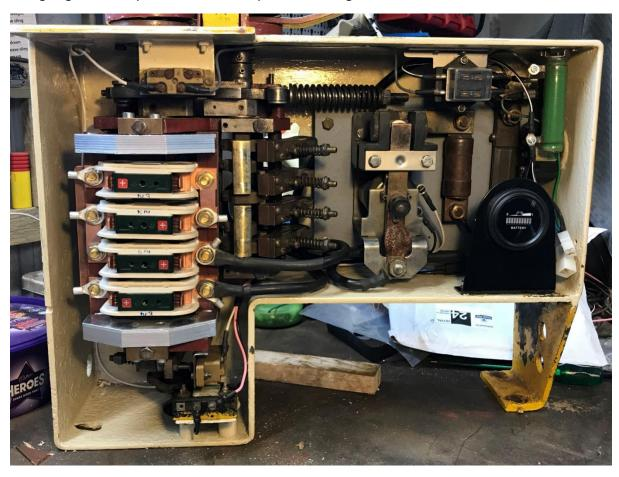
As you can see it is looking quite together and the best it has been in many years, the most recent parts completed are the switch terminal post links that I have cut and filed to shape from 1/8" copper plate. In the picture above you can also see the brass terminal nuts, on each of the four switches, holding the links and empty cable terminals (these take the place of the actual cables from the motor and resistor on the locomotive) they are there to ensure there is enough thread on each bolt.
